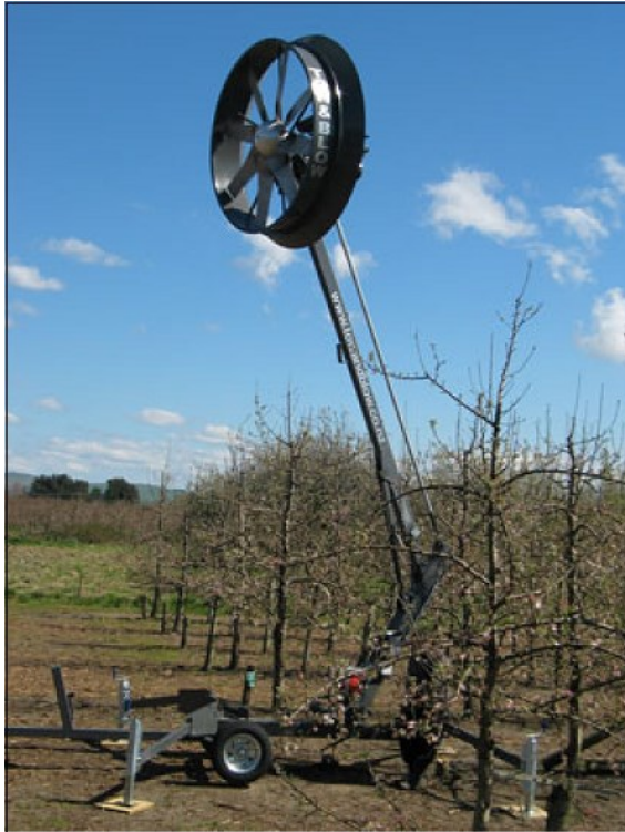
A towable wind machine for frost protection
