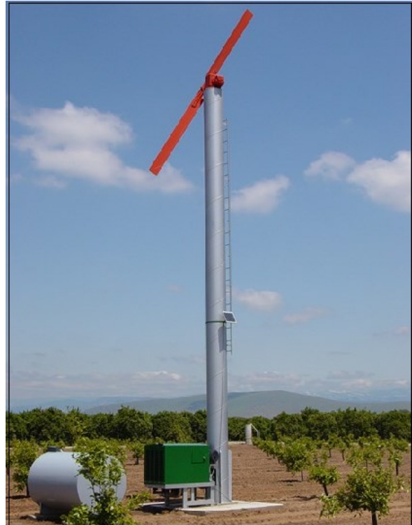
Typical wind machine for frost protection
